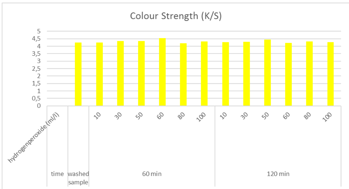
Figure 8 Color strength of bleached coconut charcoal fibers with hydrogen peroxide
