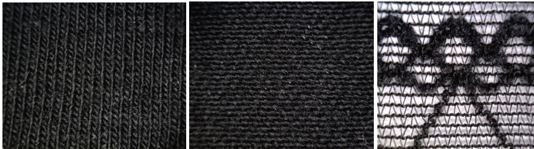
Figure 3: Yarn flow in jersey knitted structure used for the production of a bodysuit (student pictures)
