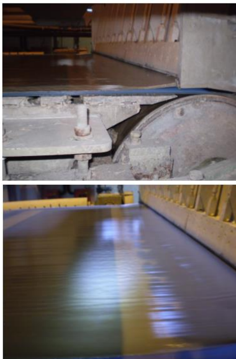
Figure 9. Surface and layout of the lower sieve on the paper machine
